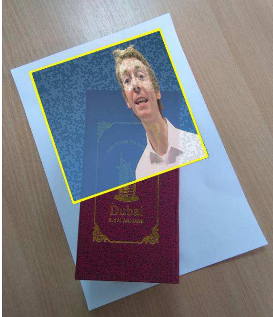
FIGURE 2. Playing YouTube video in the AR-marker area (the video's URL was decoded from the QR code which was incorporated into the AR-marker)
